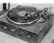
Fig. 7. The electric turntable on its simple mounting, showing control panel with switches.
