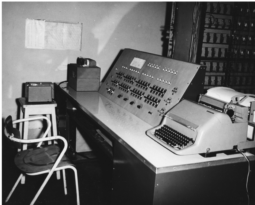
Fig. 1. The only surviving photo of the Manual Control Panel of the 1957 MR
